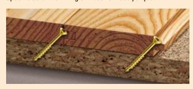
The reduced head with milling ribs and TX hexalobular recess bites into the wood without causing splitting while tightening. Head completly penetrates into the wood to allow the interlocking of the next strip. The TX recess transmits all the screwing force and prevents slipping and wear in the recess.
