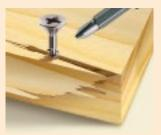
Screwing with traditional chipboard screw without pre-boring.
