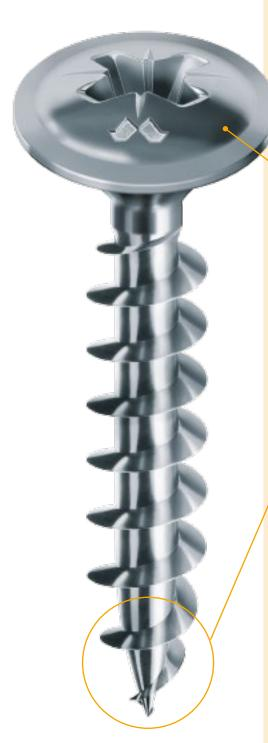
The head geometry develops a high clamping pressure making this screw particular suitable for fastening furniture back panels usually made of very soft material (thin plywood or cardboard).
