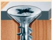
The sharp thread and narrow pitch ensure strong pull-out strength to the screw also when screwed into typically thin furniture panels.
