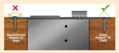
The reduced head (Ø 6 mm) allows to use a diameter screws (3,5) that guarantees better tightness, without that the head come out from the hardware.
